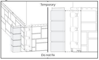
4-Install the next corner base by sliding it behind the previous one (Figure I.1) until it is supported by it (Figure I.2). Fasten the corner base on the corner of the wall and begin the second row. Repeat up to the top of the wall taking care that with each new row, the corner's height lines up with sidings. If needed, cut slightly the lower tabs to adjust the height of corner base.
