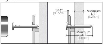
3-Never hammer the nail in completely. Leave a gap of 1/16"(0,16cm) (Figure 2).
