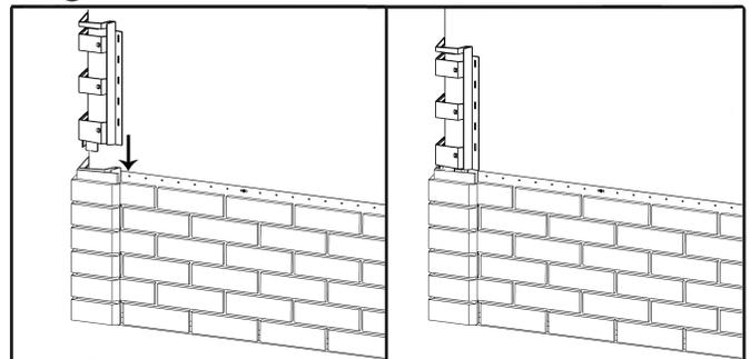
Tip: Firmly position the clips in their sockets and push evenly with both hands on the front edge of the corner.
