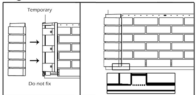
4- Install the next corner base by sliding it over the first until it is supported by it. (Figure H). Fasten the corner base on the corner of the wall and begin the second row. Repeat up to the top of the wall taking care that with each new row, the corner's height lines up with coverings (Figure I).
