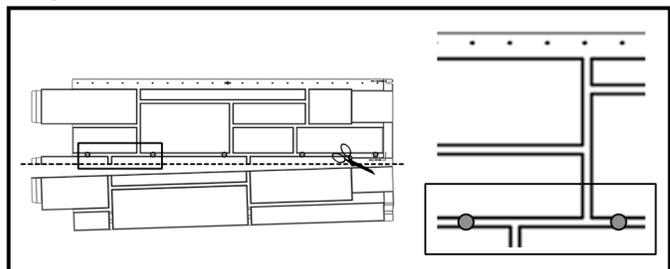
6- Repeat step four and five with succeeding panels and rows. ing the first panel with 16" increment from the cutting line of the first row. To eliminate stacking seams, alternate the cut positions for the following rows. (Figure E) (see siding installation guide for more detail)
