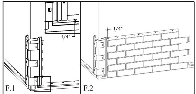
2- Install a first corner base on corners of two adjacent walls. Leave a space of about 1/4" between the bottom of the corner base and the starter strip. (Figure F.1) Slide in the first panels of a row at a distance of 1/4" from the corner base. This will allow for movement caused by expansion or contraction of the material. (Figure F.2)
