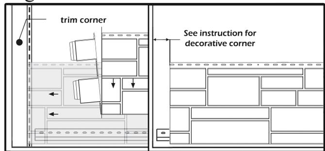
5- Install the following panel at the proper spacing according to the outdoor temperature (Figure E)(see siding installation guide for more detail).Nail in the center hole and in the installation holes.
