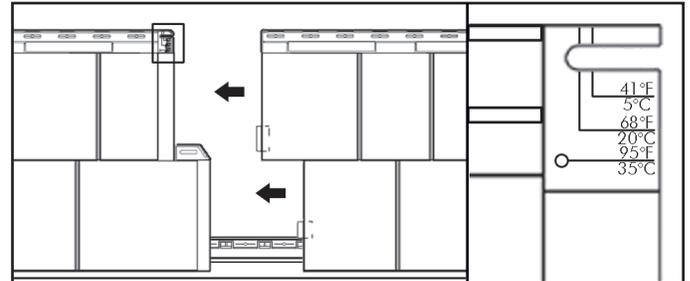
5-Begin the second row by cutting the first panel with 16"(40,64cm) increment from the cutting line of the first row. Hooking the lower panel section with the top hooks of the last installed row. To eliminate stacking seams, alternate the cut positions for the following rows. (Figure E)
