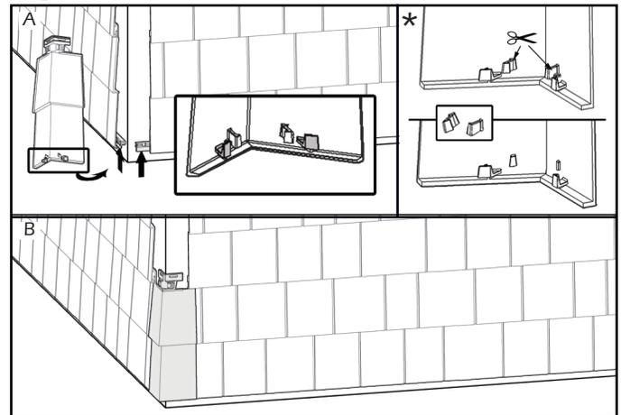
3-For all the other corners, insert the two internal hooks into the two openings (A). Ensure they are locked in place by pushing firmly near hooks to fully engage the corners. Push corner upwards on siding shingles until proper fit (B). Nail into the slots at the top (Figure H).
