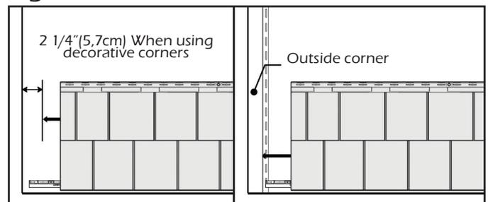
3-On each panel, hammer a nail into the center hole of the panel, this will ensure even movement of panel in both directions during expansion/contraction. Also hammer a nail into the last hole on both ends, into the lateral hole and 2 other nails into nailing channel (Figure C). Each full length panel should be secured with a minimum of 6 nails. If the panel is installed on a furring wall, a furring strip is required behind these holes.
