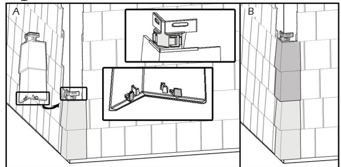
4-For the last corner only, cut excess from part. On each side of the corner, make a hole wider than the shaft of the nail, but smaller than the head. Affix a nailing strip behind these locations to fasten corners firmly. Fold back the top of the corner and nail it down. (Figure I)
