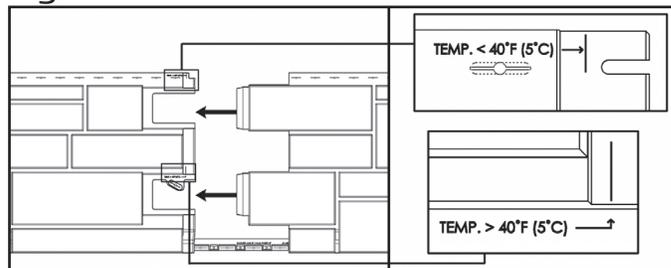
5-Start the second row by cutting the first panel with 16”(40,6cm) increment from the cutting line of the first row. Slide the hooks located at the bottom of the panel into the top of the previously installed row. (Figure E) Proceed with this row and subsequent ones following steps 3 and 4 taking care with each new row to alternate the position of the cut on the first panel. Be sure to finish one wall before beginning another.
