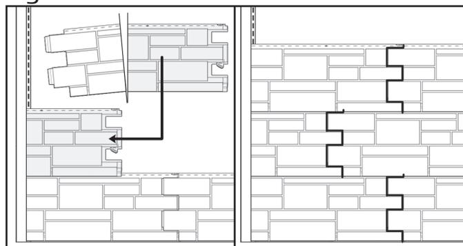
6-For the last row or places where you may need to attach siding other than in installation holes at a concealed spot on the panel use a knife to create new 1/2”(1,27cm) slots; the slot must be wider than the nail but not as wide as the nail head. (Figure F) Although not set in installation holes, this type of cutting will allow the expansion/contraction movement of siding.
